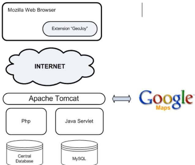
Figure 2: Basic semi-automatic geocoding system architecture
