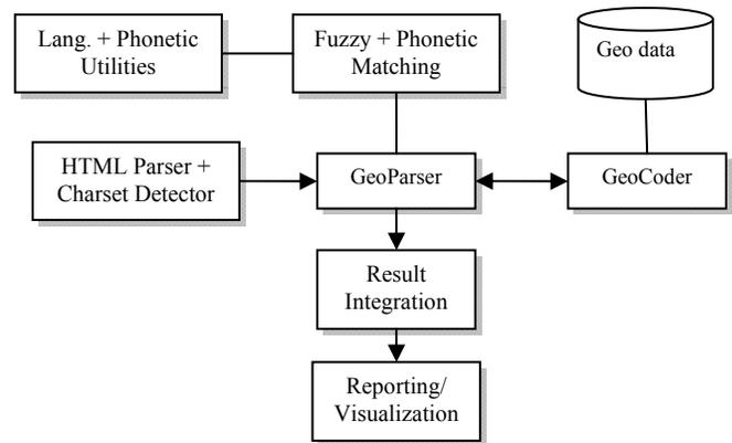
**Figure 1: Automatic geocoding system architecture**
