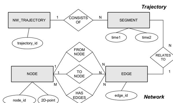
Figure 1: A conceptual schema for modeling trajectories exploiting the network aspect
