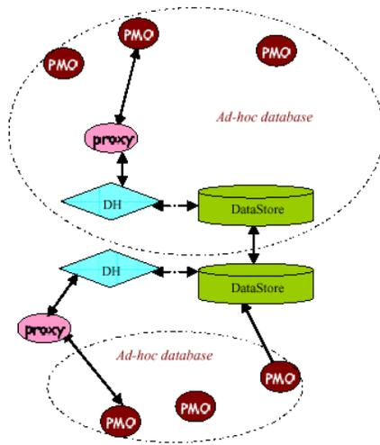
Figure 1: DB-Globe system architecture [10], [13]
